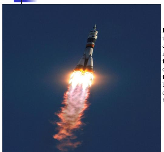
Rocket propellant is mass that is stored, usually in some form of propellant tank or casing, prior to being used as the propulsive mass that is ejected from a rocket engine in the form of a fluid jet to produce thrust. For chemical rockets often the propellants are a fuel such as liquid hydrogen or kerosene burned with an oxidizer such as liquid oxygen or nitric acid to produce large volumes of very hot gas.
