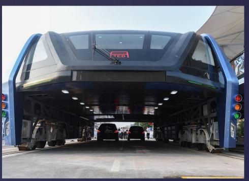
The "straddling bus" would roll on stilts above traffic using small tracks positioned between lanes of traffic while passengers get on and off at elevated bus stops. The result: additional people carrying capacity for urban roads, no disruption to traffic and no need to build completely independent track systems. Seems like a win/win, but at this stage we're not aware of any progress on the expected pilot program.
