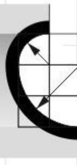
A technical diagram showing the profile of a skocia. It is an asymmetric shape formed by two circular arcs of different radii. The upper arc is concave, and the lower arc is convex. A grid is overlaid on the diagram to show its proportions. Arrows indicate the radii of the arcs. The diagram is positioned to the left of the word 'СКОЦИЯ', which is rendered in a large, bold, black sans-serif font.
