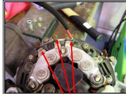
Any Of These Stator Connections Can Be Used As A W Terminal. Solder An Insulated Wire Onto The Terminal To Use As The Tacho Signal
