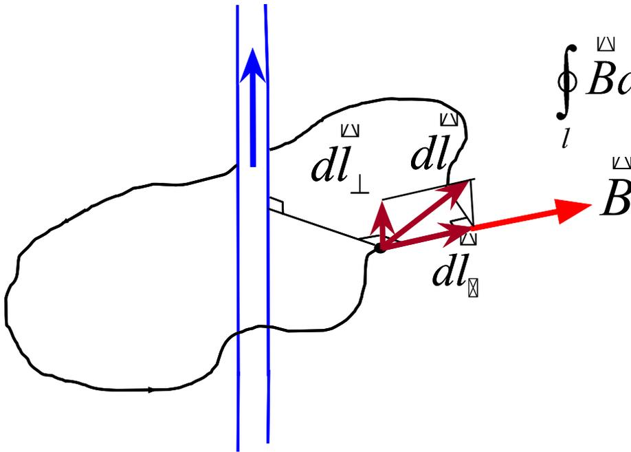
$$d\vec{l} = d\vec{l}_{\perp} + d\vec{l}_{\parallel}$$
