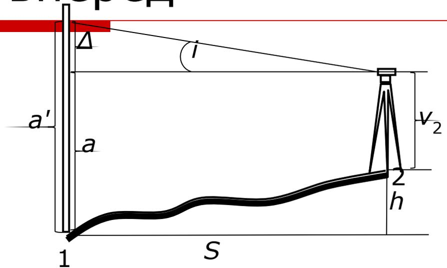
$$h = a - v_2 = a' - \Delta - v_2$$
