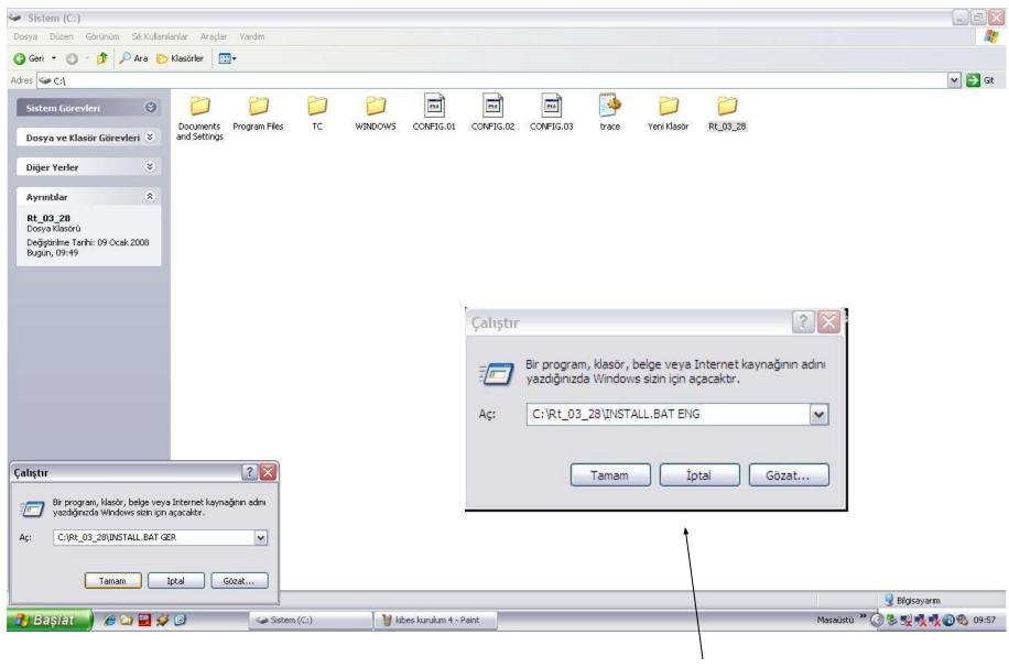
Press space and write ENG to the end of the command (C:\Rt\_03\_28\INSTALL.BAT) that is shown on screen.
