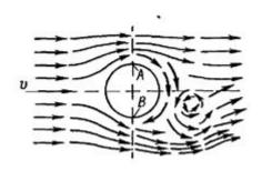
Wire vibration occurs at wind speeds of 0.6–0.8 m / s; when the wind speed increases, the vibration frequency and the number of waves in the span increase, and when the wind speed exceeds 5-8 m / s, the vibration amplitudes are so small that they are not dangerous for the wire.
