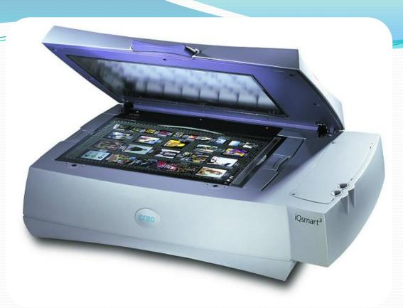
Flatbed scanners - the most common type of scanner because it provides maximum comfort for the user high quality and affordable scanning speed. It is a tablet, inside of which is located under the transparent glass scanning engine.
