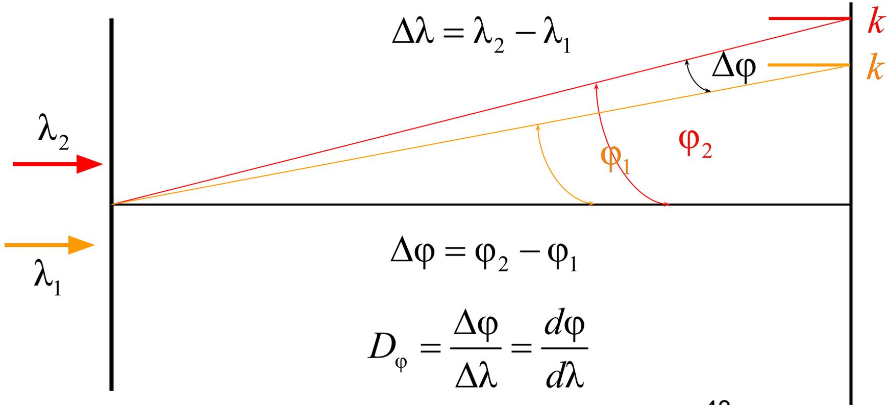
$$\lambda = \frac{d}{k} \sin \varphi \qquad \frac{d\lambda}{d\varphi} = \frac{d}{k} \cos \varphi$$
