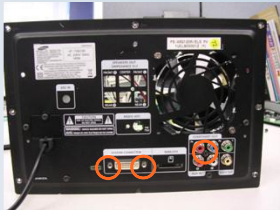
3. Unfasten System Cable Screw(2 places) with (-) driver. 4. Unfasten screw (1 place) of the Jack.
