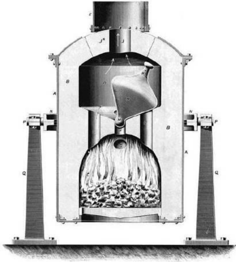
FIG. 24. BESSEMER'S FURNACE FOR THE MANUFACTURE OF OPTICAL GLASS
