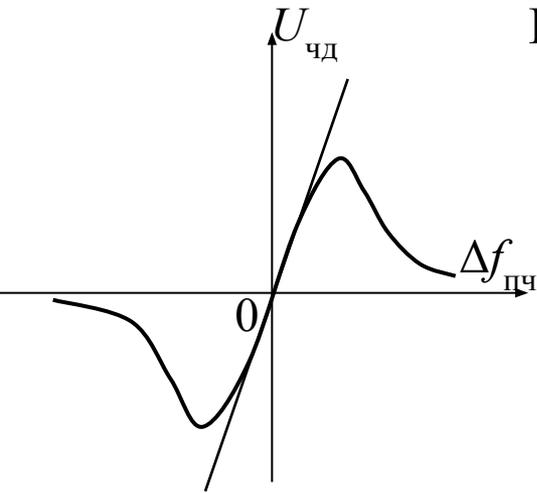
$$U_{\text{чд}}(\Delta f_{\text{пч}}) \rightarrow K_{\text{чд}} \Delta f_{\text{пч}}$$
