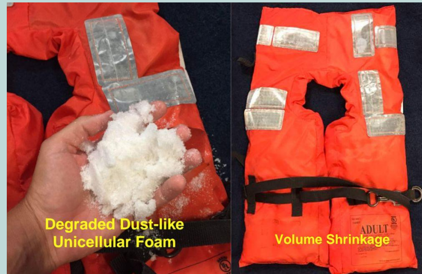
Deteriorated life jackets
