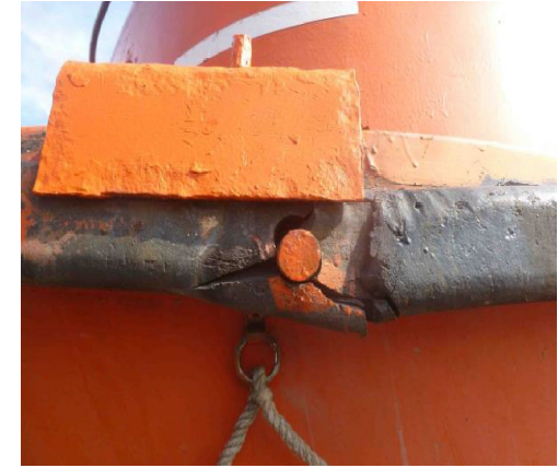
Fractured fender for life boat.
