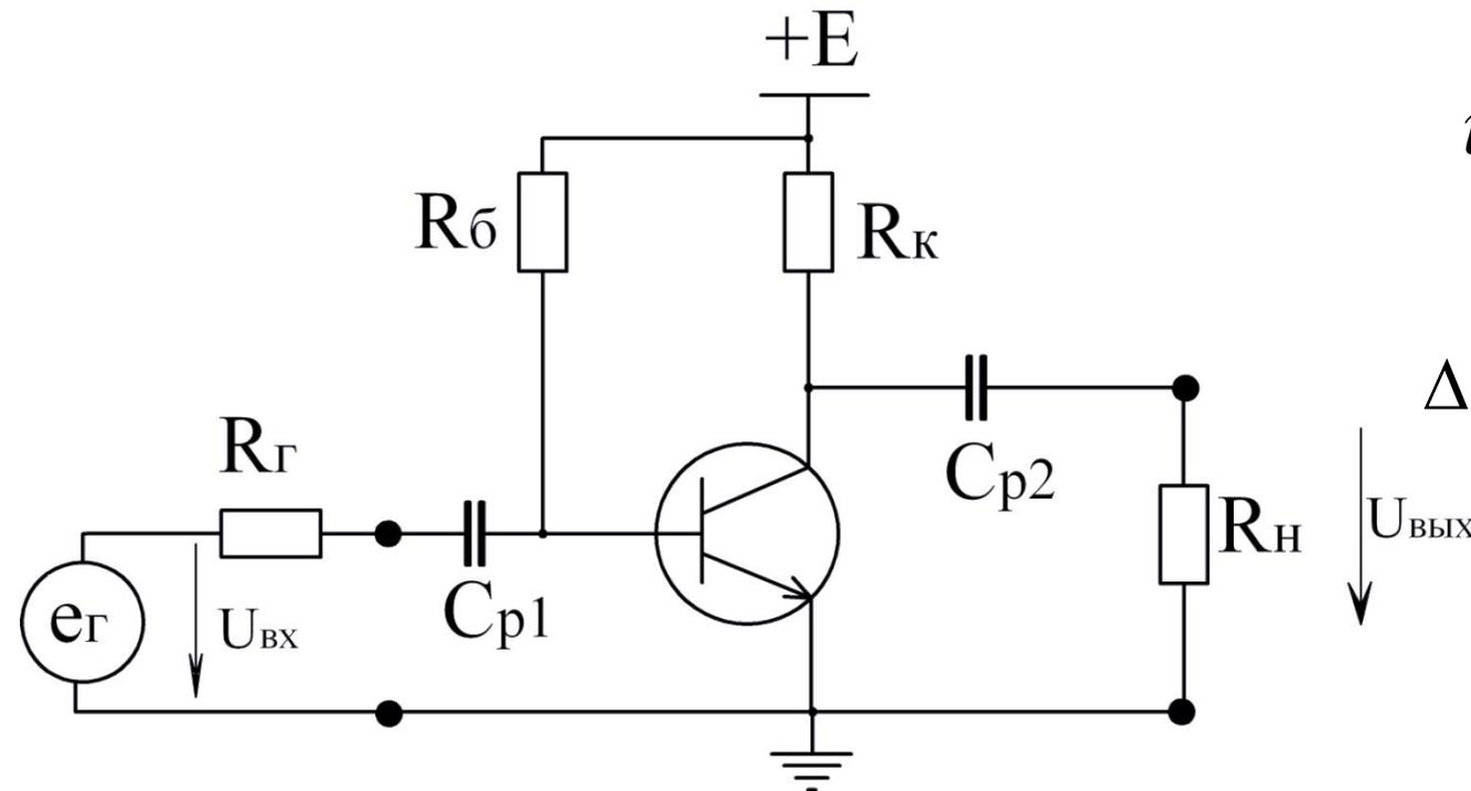
$$u_{\text{вых}} = R_{\text{H}} \cdot i_{\text{K}}$$
