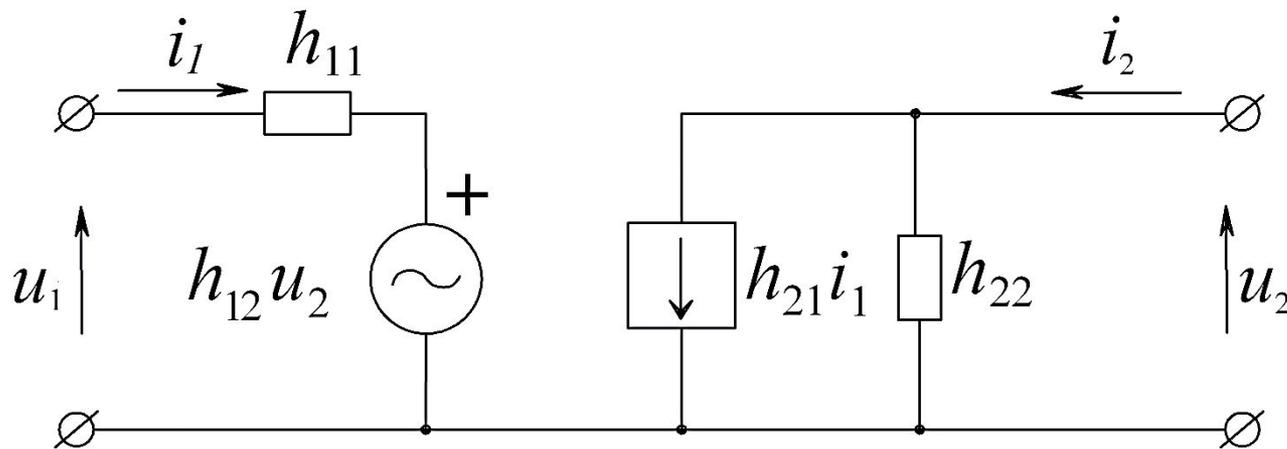
$$dU_1 = \frac{\partial U_1}{\partial I_1} dI_1 + \frac{\partial U_1}{\partial U_2} dU_2, \quad u_1 = h_{11}i_1 + h_{12}u_2$$
