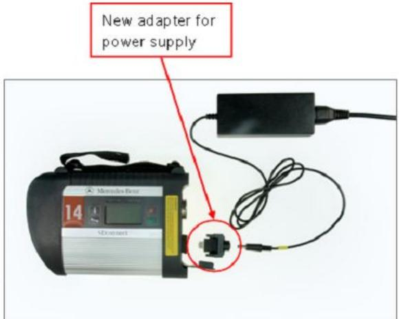
Plug in power supply cable directly into adapter's socket.
