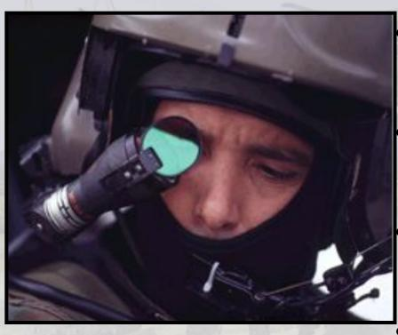
Display provides unobstructed imagery for pilotage and targeting
