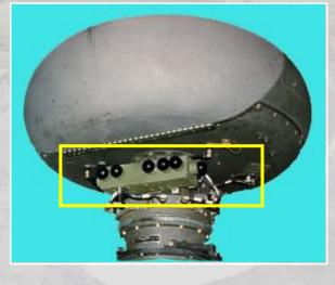
Radar Frequency Interferometer (RFI)
