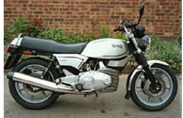
Norton Classic air-cooled twin-rotor motorcycle
