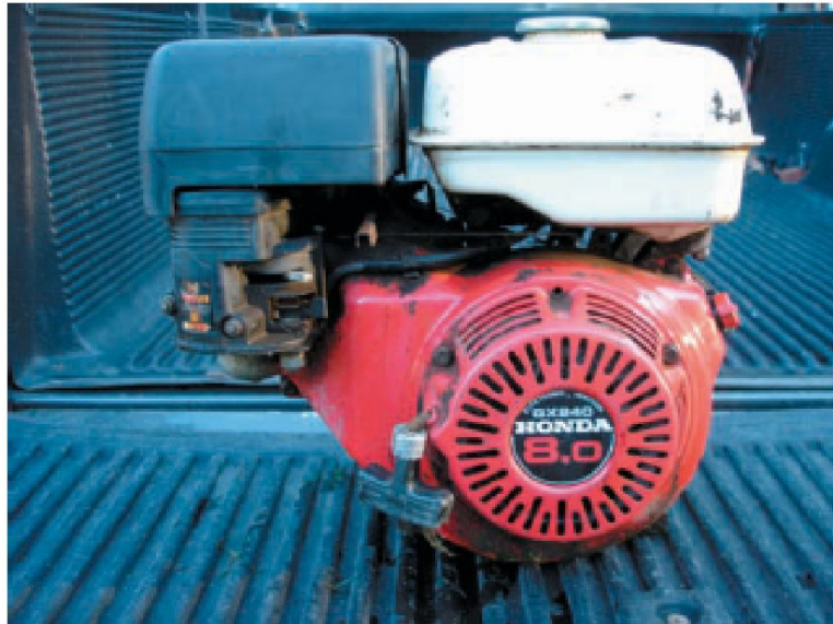
Figure 4 A typical fuel tank. Note that the fuel tank is placed higher than the carburetor and therefore uses a gravity feed system.
