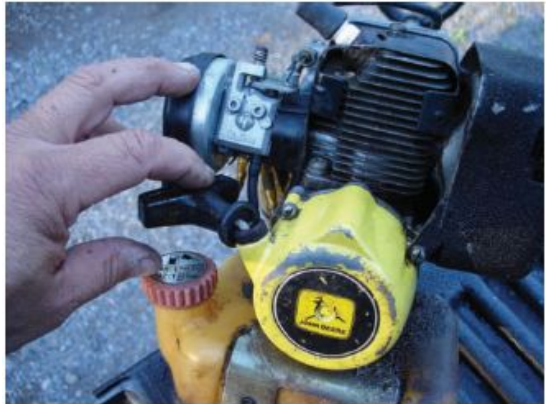
Figure 29 A diaphragm carburetor can be turned in any angle without impairing operation
