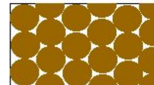
tightly packed, uniform particle size
