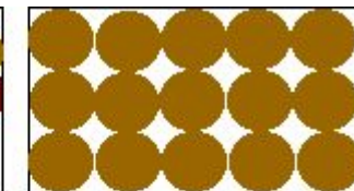
loosely packed, uniform particle size
