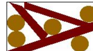
loosely packed, well structured material
