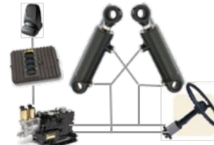
Flow amplifying series with steering pilot Orbitrol
