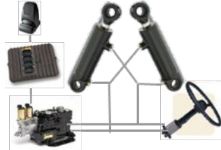
Joystick steering Parallel with steering Orbitrol
