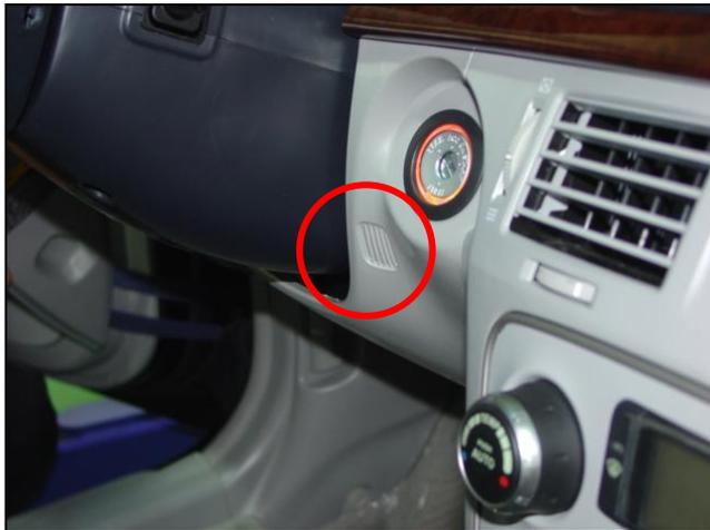
Humidity sensor detects the relative humidity of the car's cabin. This sensor converts it into the voltage signal and sends the signal to the FATC controller.
