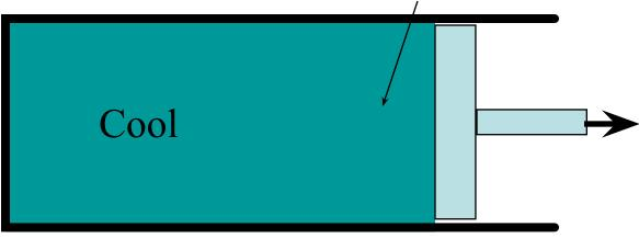
When the gas is compressed it heats up. The compressor compresses the gas and removes heat of compression.
