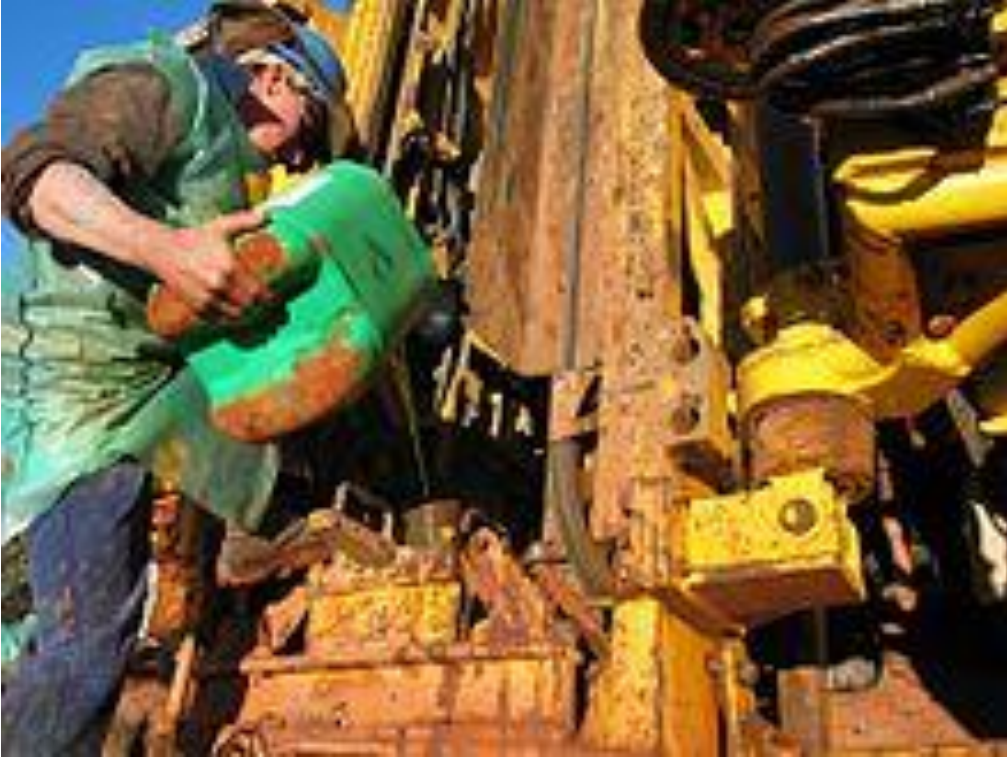
Driller pouring anti-foaming agent down the drilling string on a drilling rig
