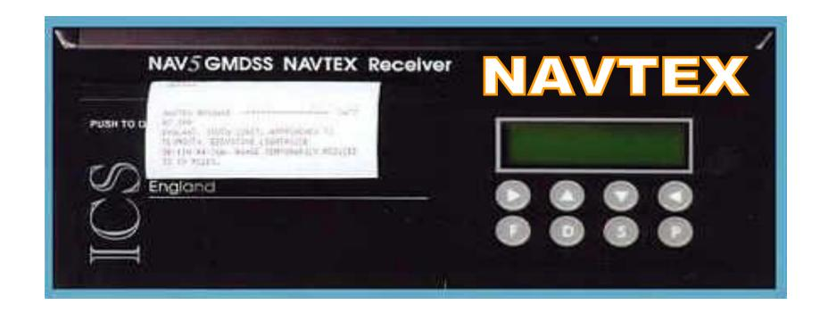
NAVTEX is a telex-receiver/printer installed on GMDSS-vessels to receive *Maritime Safety Information-messages* (MSI). These navigational messages are addressed "to all vessels" and contain information concerning meteorological warnings, SAR-operations and other important and urgent data.
