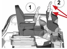
**Override Buttons** located on the front of the joystick controls.
