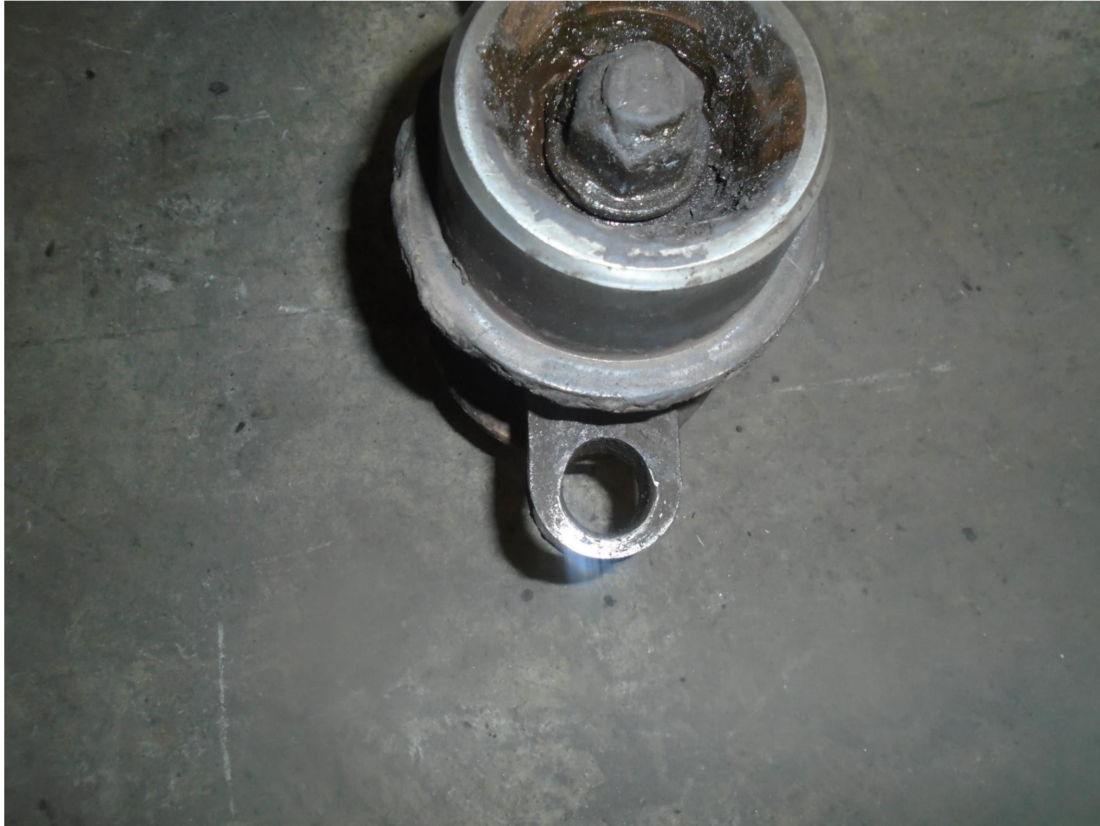
Elevator chain link's pin hole badly worn out
