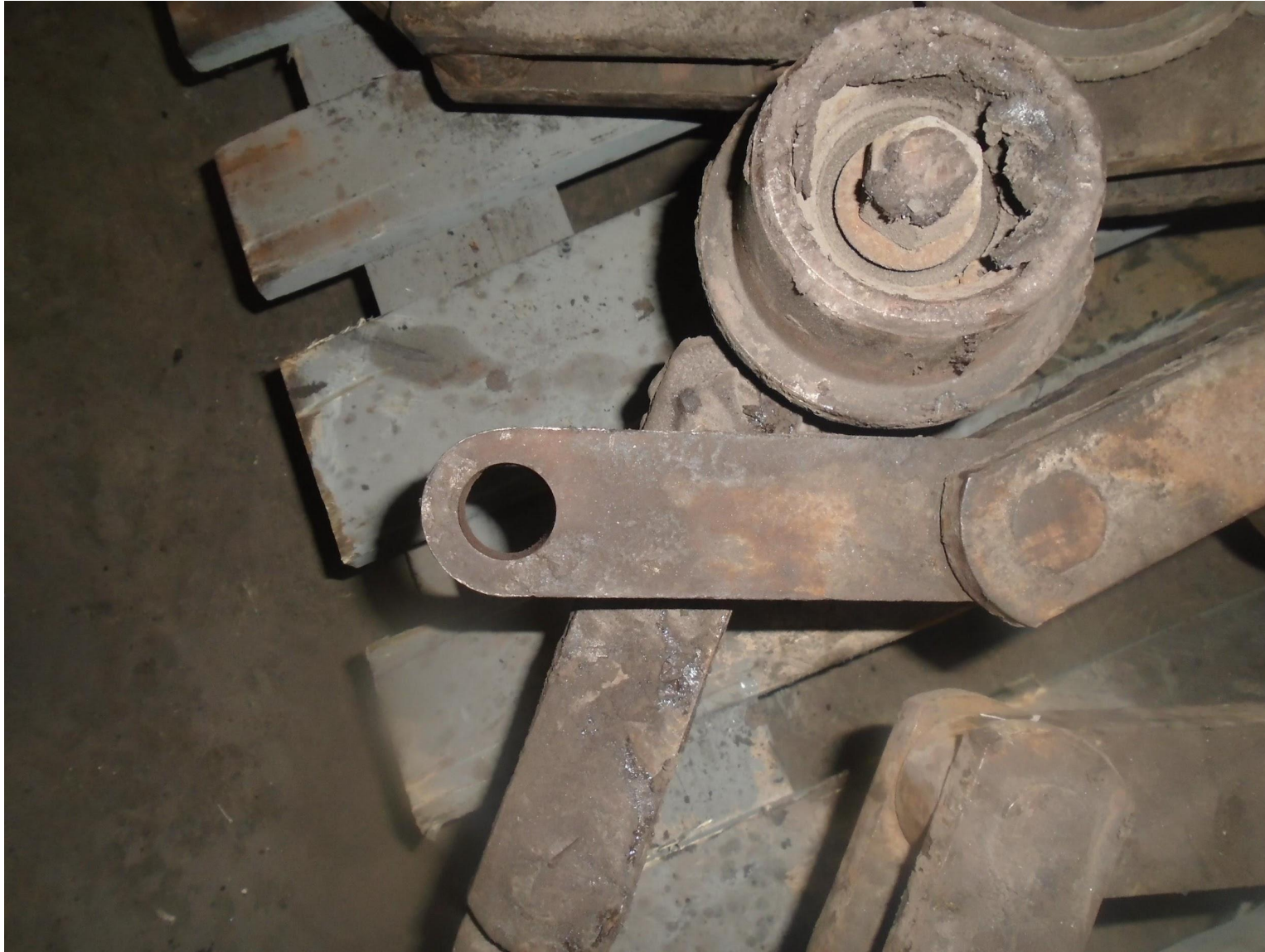
Elevator chain link's Pin hole worn out
