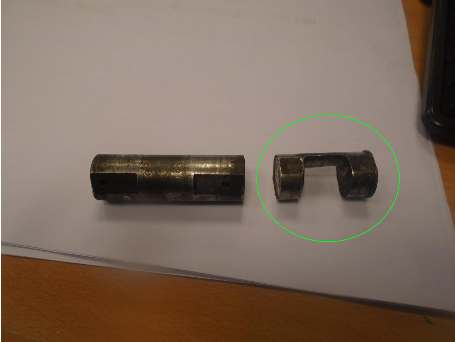
Elevator chain link's pin badly worn out
