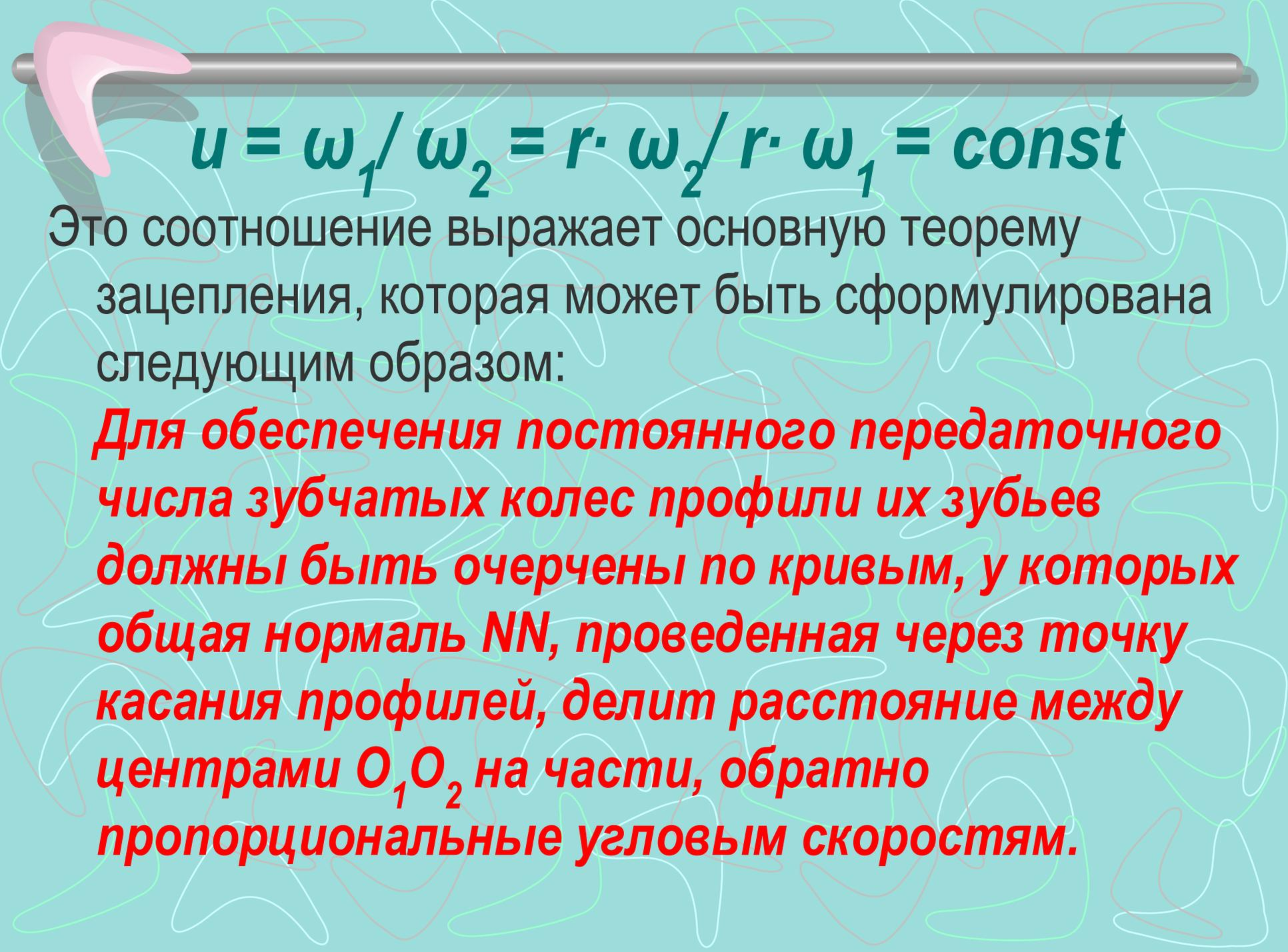
$$u = \omega_1 / \omega_2 = r \cdot \omega_2 / r \cdot \omega_1 = \text{const}$$
