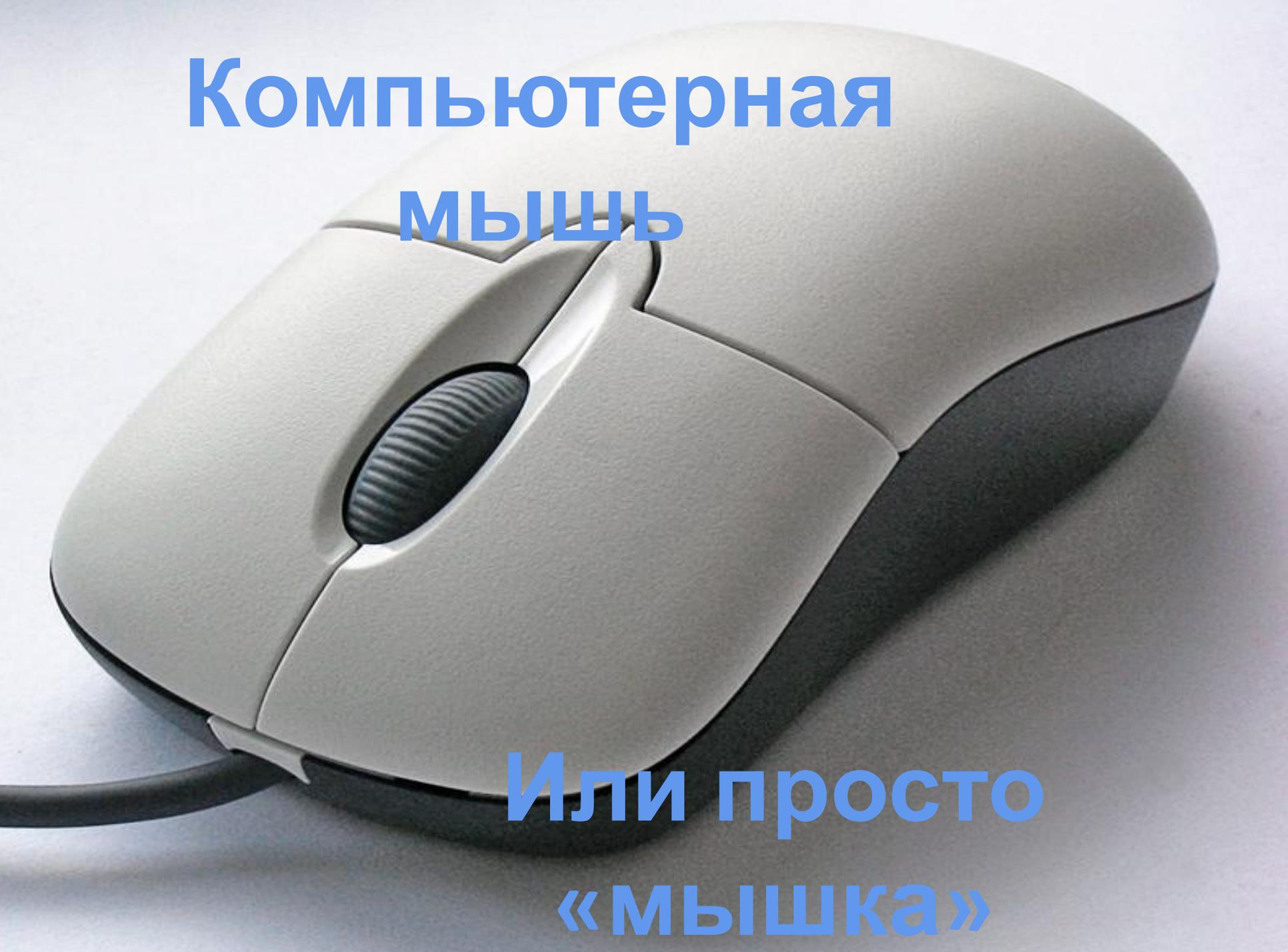
A white computer mouse with a scroll wheel and two buttons. The mouse is shown from a three-quarter perspective, highlighting its ergonomic design. The scroll wheel is a dark grey color with a ribbed texture. The mouse has a cord attached to the bottom left.
