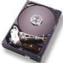
A 3.5-inch hard disk drive, shown from a top-down perspective, revealing the internal platters and read/write head.                                                         |              |
