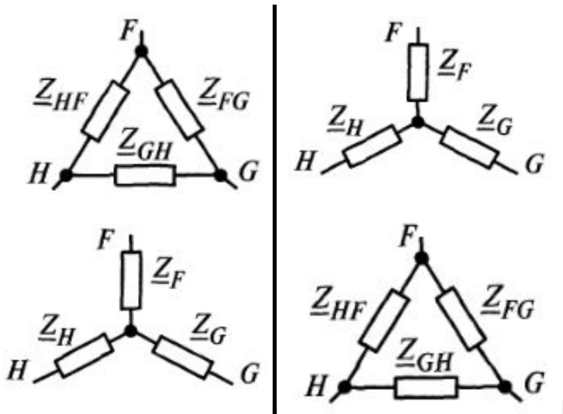
$$\underline{Z}_F = \frac{\underline{Z}_{FG} \underline{Z}_{HF}}{\underline{Z}_{FG} + \underline{Z}_{GH} + \underline{Z}_{HF}}$$
