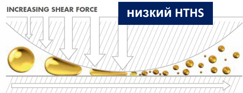
FIGURE 1a: An engine oil with low shear stability breaks down under high stress.
