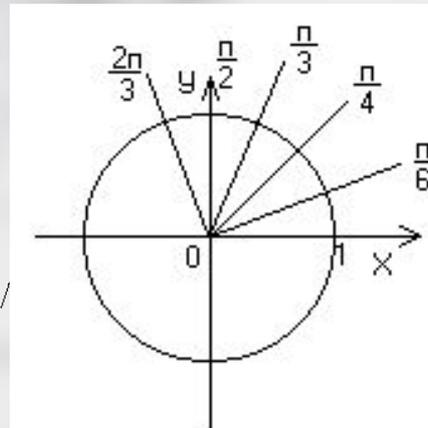
$$\begin{aligned} 0 &= 0^\circ \\ \pi / 6 &= 30^\circ \\ \pi / 4 &= 45^\circ \\ \pi / 3 &= 60^\circ \\ \pi / 2 &= 90^\circ \\ \pi &= 180^\circ \end{aligned}$$
