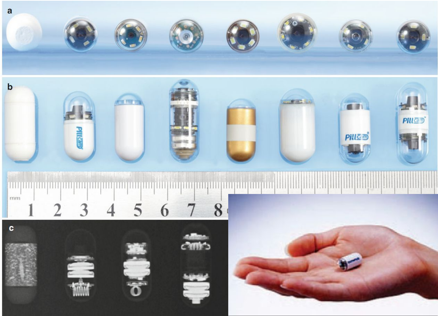
Fig. 3.1 Front view (a) and top view (b) of the capsules, with corresponding X-ray image (c). Left to right: Agile patency capsule, PillCam SB2, EndoCapsule, CapsoCam, MiroCam, OMOM capsule, PillCam ESO2, PillCam COLON2
