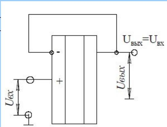
$$R_{\text{БХ}} = R_{\text{БХ}0} (1 + K_{U0}); R_{\text{БЫХ}} = \frac{R_{\text{БЫХ}0}}{(1 + K_{U0})}$$
