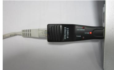
Connect USB Ethernet Cable to PC USB Port.
