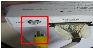
Connect GND cable to JIG
