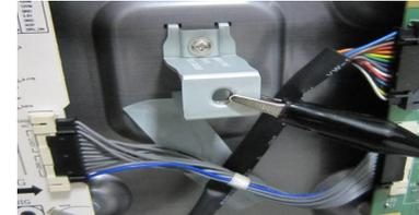
Connect JIG GND cable to the T-Con Board GND.
