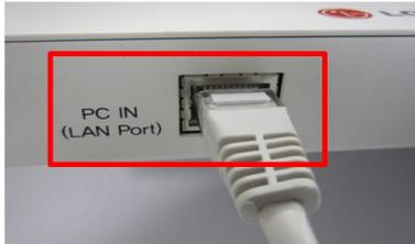
Connect LAN Cable to JIG PC IN(LAN Port)
