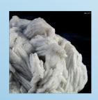
**Barite**  $BaSO_4$  - is determined by the tabular, prismatic and isometric forms of crystals (Figure 15), perfect cleavage, low hardness (tv. 3-3.5) and high density (4.5 g/cm 3).
