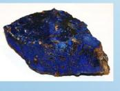
Azurite  $Cu_3[CO_3]_2(OH)_2$  - is determined by the bright blue color, shape of aggregates - small tabular crystals, druses, brushes, radially fibrous, nodules, solid grainy and earthy aggregates (Figure 15); easily decomposed in HCl.
