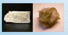
Gypsum  $CaSO_42H_2O$  - pure gypsum is colorless transparent or snow-white, has flattened crystals, very perfect cleavage, low hardness (easily scratched with a fingernail), does not react with hydrochloric acid.
