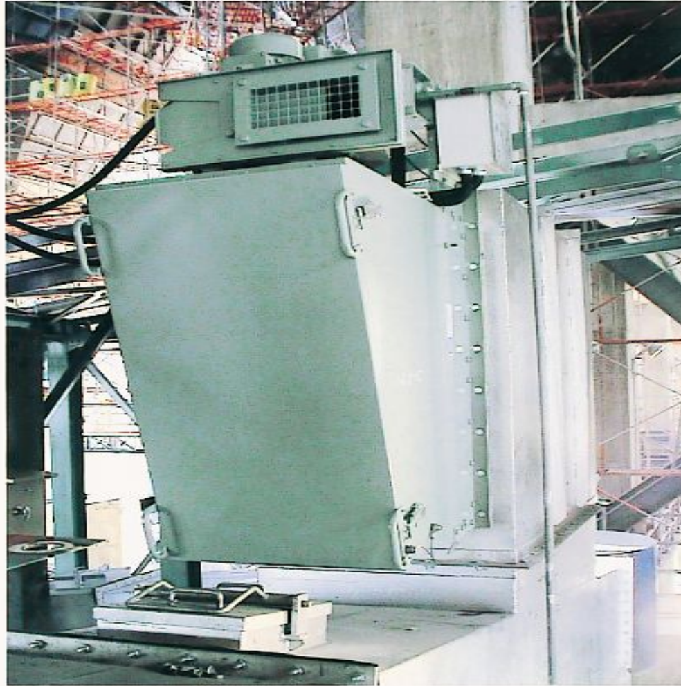
Application: Raw meal air slide Material: Raw meal. Type: DLM V 18/15 H.
