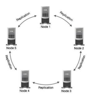
In Cassandra, replicas for a given piece of data are distributed on one or more of the nodes in a cluster. If it is detected that some of the nodes responded with an out-of-date value, Cassandra will return the most recent value to the client. After returning the most recent value, Cassandra performs update of the stale values in the background: process known as **read repair**.
