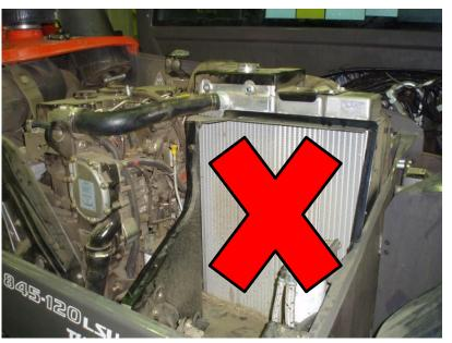
Service points not logically grouped and located deep into the engine compartment
