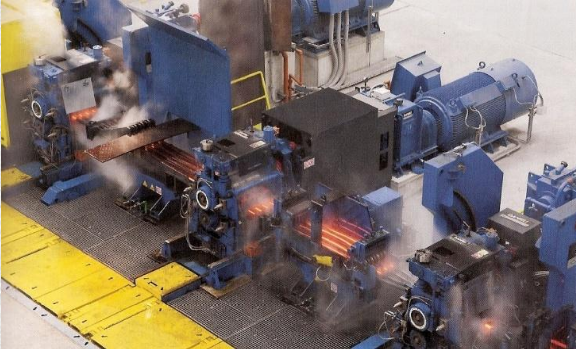
Fig.5 Multi-slitting rolling in the finishing group of stands.
