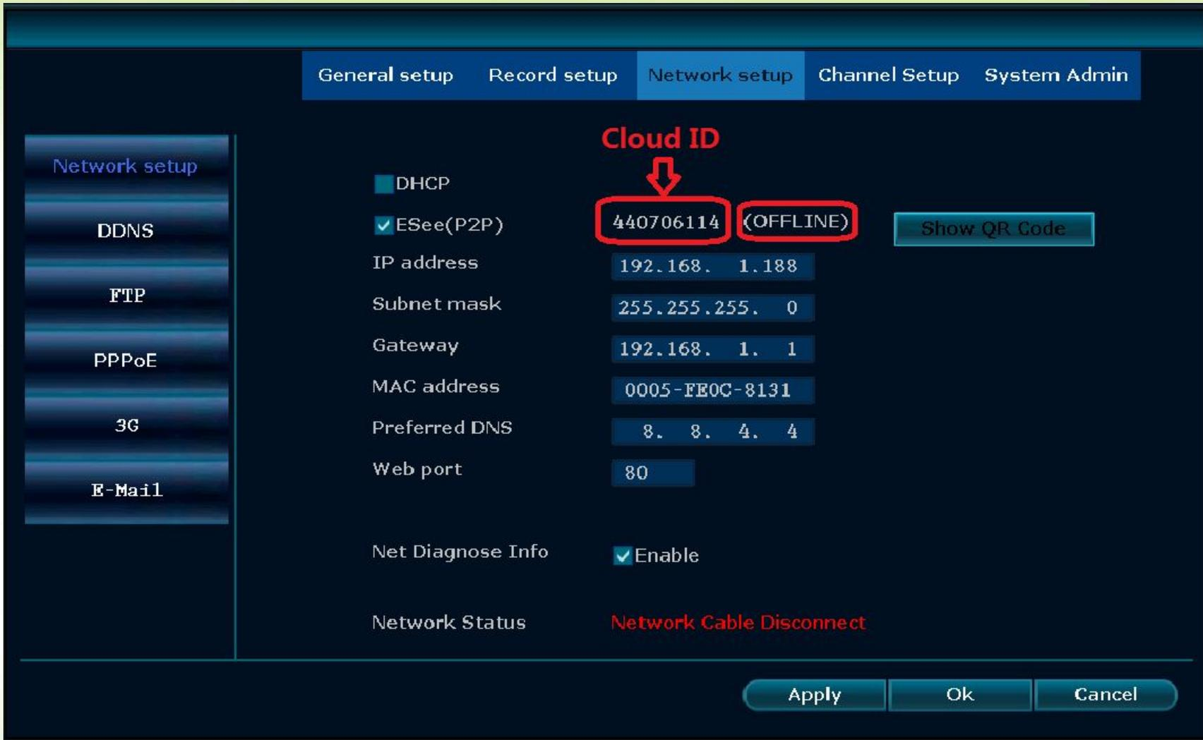
The screenshot shows the 'Network setup' menu of an NVR. The 'Cloud ID' is highlighted with a red box and a red arrow pointing to it. The status is '(OFFLINE)'. A 'Show QR Code' button is visible next to the Cloud ID. The network status at the bottom indicates 'Network Cable Disconnect'.
