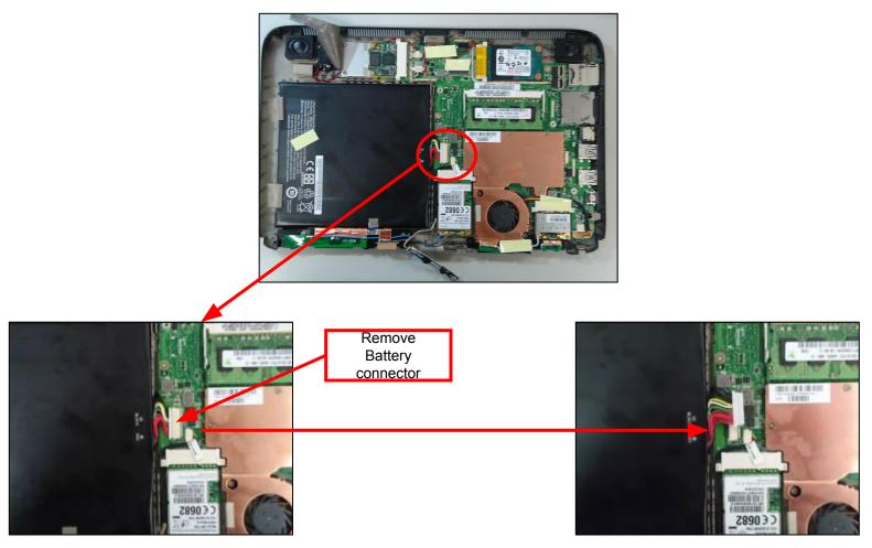
Remove key part before requirement remove battery connector for safety.
