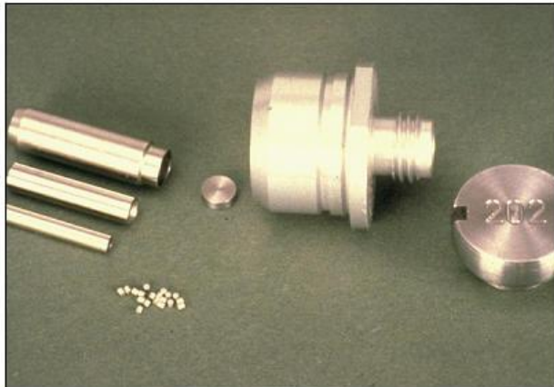
Cobalt 60: Radiation source for the Gamma Knife ®
