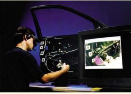
Augmented Reality can be used for training as well as for assembly purpose
