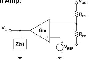
$$\frac{V_{\text{OUT}}}{V_{\text{OUT}}} = -\frac{R_{\text{F2}}}{R_{\text{F1}} + R_{\text{F2}}} \bullet \text{Gm} \bullet Z(s)$$
