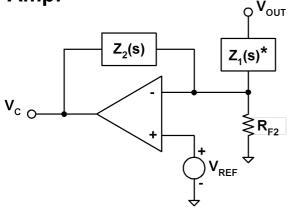
$$\frac{V_{C}}{V_{OUT}} = -\frac{Z_{2}(s)}{Z_{1}(s)}$$
