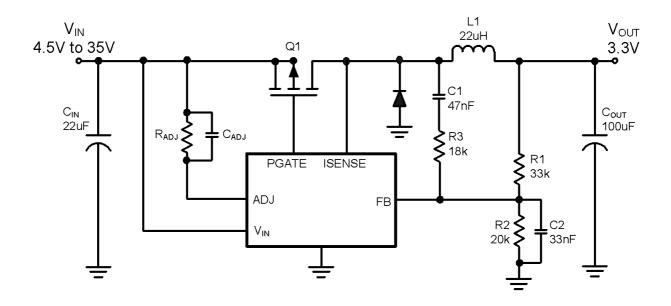
$C_{OUT}$  has excessive ESL, so  $\Delta V_{OUT}$  has large voltage steps that result in erratic switching. C2 filters-out ESL voltage step at FB pin. C1, C3 and R3 generate triangle waveform that determines the switching frequency.
