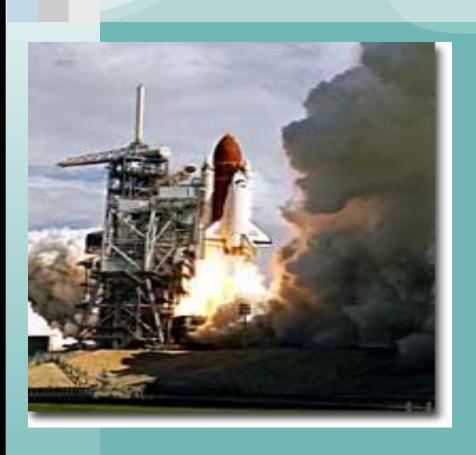
Space shuttle's rocket boosters propel the orbiter into space by exerting an equal and opposite force to exhaust gasses.
