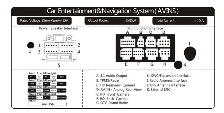
3. Connect the cable based on No. in below pictures. original car cables plug into the corresponding plug of the Car Pad 4.
