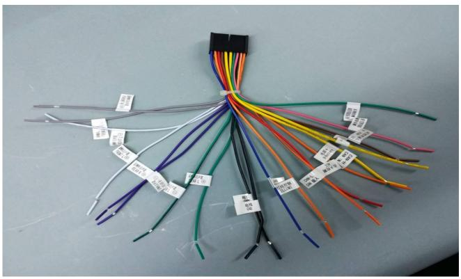
Amplifier cable (support  $2\Omega$  or  $4\Omega$  speaker) Max output:50W\*4;
