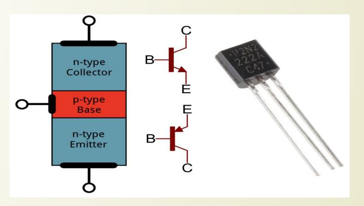
Transistor is a semiconductor element of a chip. Depending on the order of the semiconductor layers, transistors are divided into NPN and PNP types.
