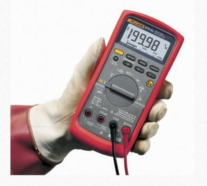
Ammeter (from ampere  $+ \mu \epsilon \tau \varrho \dot{\epsilon} \omega - I$ measure) is a device for measuring current in amperes. The ammeter scale is graded in microamperes, milliamperes, amperes or kiloamperes in accordance with the measurement range of the instrument.
