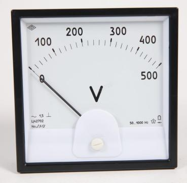
An ideal voltmeter should have an infinitely large internal resistance. Therefore, the higher the internal resistance in a real voltmeter, the less influence the device has on the measured object and, consequently, the higher the accuracy and the more diverse the field of application. Voltmeters are connected to the network in parallel.
