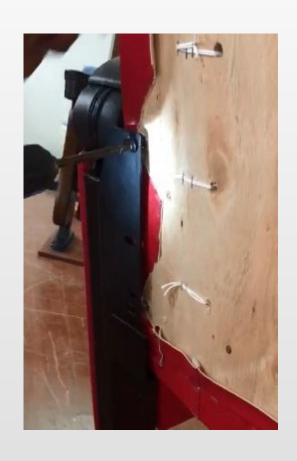
4. Step 4.Install the chair seat, Use a kind of wrench like this, to ajust the center metal at the seat. This step it is so important. If installed not well. It can not folding.
